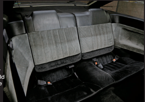
To ensure head clearance for occupants, the ceiling has a contoured shape.
