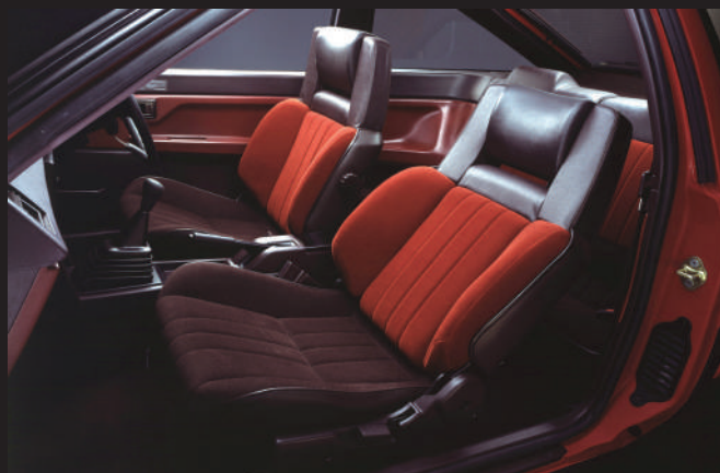
The sports seats feature adjustable side support. By gripping the pump located on the left side of the seat, the driver can adjust the lumbar support.
