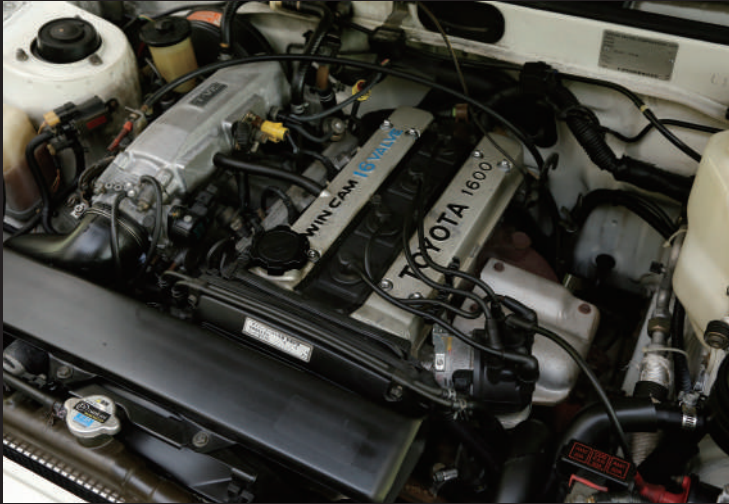
Equipped with the newly developed 4A-GEU DOHC engine, featuring 4 valves per cylinder for a total of 16 valves.
