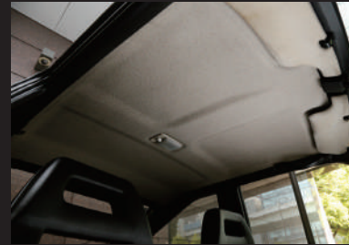
To ensure head clearance for occupants, the ceiling has a contoured shape.
